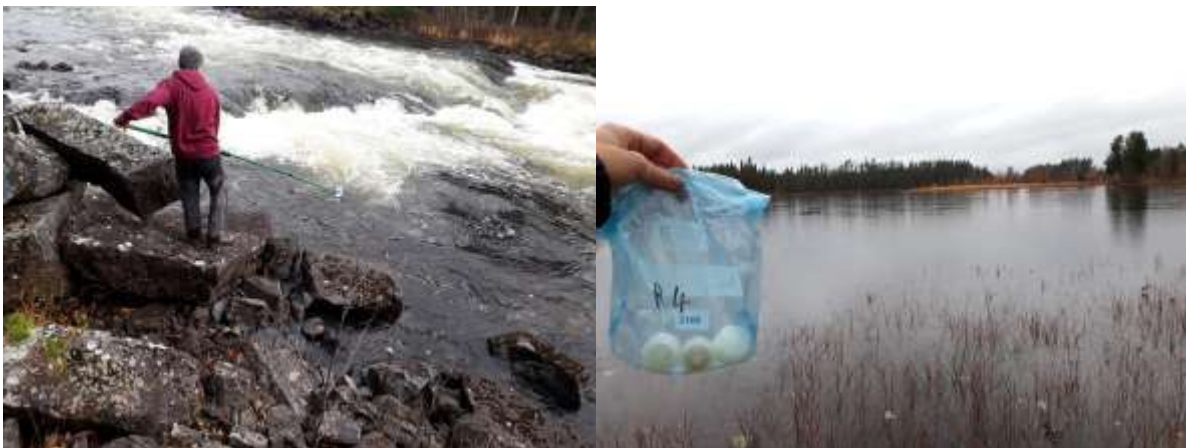
Figure 1: Water sampling directly from the free-flowing water (left) and three glass fiber filters after water sampling (spot R004, Rörströmsälven) (right).
